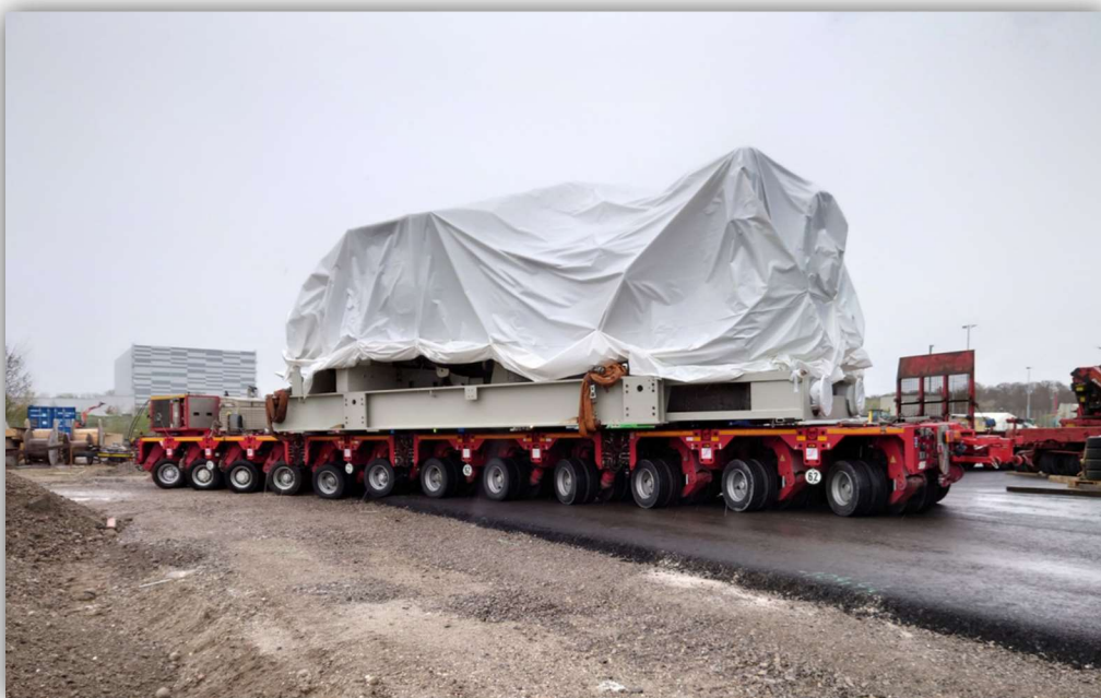
Gas turbine – turbine being transported to ware house
